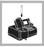
**9.** Place the sample vial into the adapter with the Hach logo facing the front of the instrument. Close the light shield. Results in mg/L COD (or chosen units) will be displayed.
