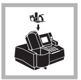
**4.** Insert the Test 'N Tube Adapter into the sample cell module by sliding it under the thumb screw and into the alignment grooves. Fasten with the thumb screw.
