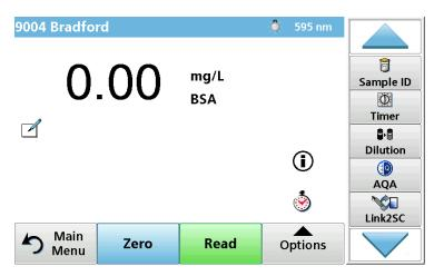
Start the program with the measurement of the blank value (buffer). Insert the cuvette and press **Zero**.
