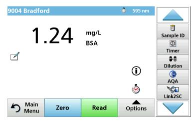
Then add the sample to the cuvette and measure the sample by pressing on **Read**. The result is shown in the display as **mg/L BSA**.
