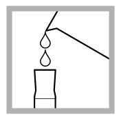
**4.** Use a graduated cylinder or TenSette pipet to measure the sample volume from Table 2 on page 3.
