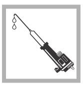
**3.** Hold the Digital Titrator vertically with the cartridge tip up. Turn the delivery knob to eject air and a few drops of titrant. Reset the counter to zero and clean the tip.
