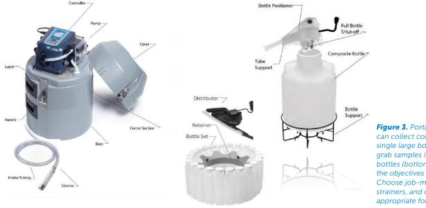
**Figure 3.** Portable automatic samplers can collect composite samples in a single large bottle (far right) or individual grab samples in a series of separate bottles (bottom center), depending on the objectives of the testing program. Choose job-matched sampling tubes, strainers, and control options appropriate for the task at hand.
