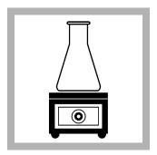
3. Boil the sample gently for 30 minutes. Do not let the flask boil dry. For the best recovery, concentrate the sample to less than 20 mL. After concentration, maintain the volume of sample near 20 mL by adding small amounts of deionized water. Do not exceed 20 mL.
