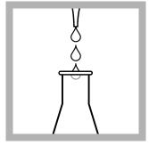
2. Add 2.0 mL of 5.25 N Sulfuric Acid Solution to the flask
