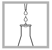
**4.** Let the sample cool to room temperature. Add 2.0 mL of 5.0 N Sodium Hydroxide Solution to the flask.
