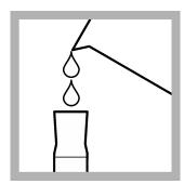
**6.** Pour the sample into a 25-mL graduated cylinder. Adjust the volume to 25 mL by rinsing the flask with deionized water and pouring the rinse water into the cylinder.
