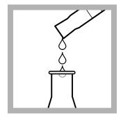
1. Use a graduated cylinder to add 25-mL of sample into the 125-mL Elenmeyer flask.
