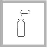
6. Add the contents of one DPD Free Chlorine Powder Pillow to the sample cell (the prepared sample). Swirl the sample cell for 20 seconds to mix. Wait 30 seconds for any undissolved powder to settle. Proceed to step 7 immediately.
