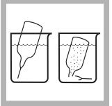
**8.** Fill a DPD Free Chlorine Reagent AccuVac Ampul with sample.
