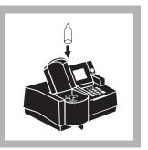
10. Immediately (within one minute of sample addition) place the AccuVac Ampul into the cell holder. Close the light shield. Results in mg/L chlorine dioxide (or chosen units) will be displayed.
