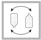
**9.** Quickly invert the ampul several times to mix. Wait 30 seconds for any undissolved powder to settle. Wipe off any liquid or fingerprints.
