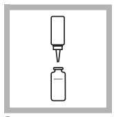
**5.** Add four drops of Glycine Reagent to the sample. Swirl to mix. This is the prepared sample.
