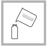
**3.** Fill a sample cell with 10 mL of sample (the blank). Place it into the cell holder and close the light shield.
