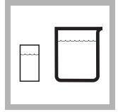
**4.** Fill a zeroing vial (the blank) with at least 10 mL of sample. Fill a 50-mL beaker with 40 mL of sample.
