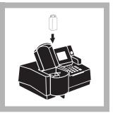
7. Place the prepared sample into the cell holder. Close the light shield. Read results in mg/L chlorine dioxide (or chosen units) within one minute of reagent addition.
