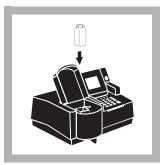
**16.** Place the prepared sample into the cell holder. Close the light shield. Results in mg/L total kjeldahl nitrogen as N (or chosen units) will be displayed.
