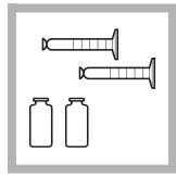
**13.** When the timer beeps, pour the contents of each cylinder into separate 25-mL sample cells.
