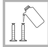
**10.** Fill both cylinders to the 25-mL mark with deionized water. Stopper. Invert several times to mix.
