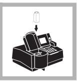
**14.** Place the blank into a cell holder. Close the light shield.
