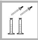
**6.** Add 1.0 N KOH to each cylinder, one drop at a time, mixing after each addition. Continue until the first permanent blue color appears.
