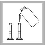
**7.** Fill both cylinders to the 20-mL mark with deionized water.
