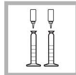
**9.** Add three drops of Polyvinyl Alcohol Dispersing Agent to each cylinder. Stopper. Invert several times to mix.
