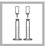
**8.** Add three drops of Mineral Stabilizer to each cylinder. Stopper. Invert several times to mix.
