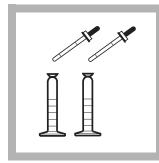
**5.** Add one drop of TKN Indicator to each cylinder. Add drops of 8.0 N KOH to each cylinder until the first flash of blue color appears. Stopper and invert the cylinder each addition.
