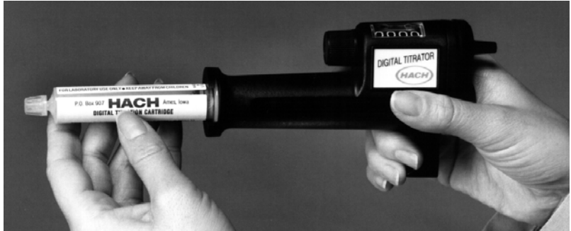
Figure 2 Sliding the Cartridge into Place
