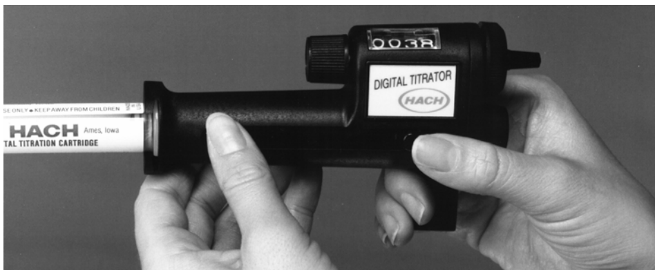
Figure 7 Retracting the Plunger
