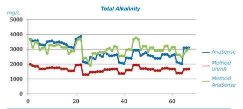
Figure 4: Comparison between the online measurements and the laboratory results at Carlsberg
