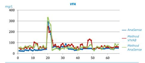
Figure 5: Comparison between the online measurements and the laboratory results at Carlsberg
