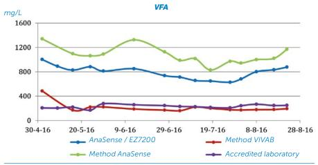
Figure 2: Comparison between the online measurements and the weekly laboratory results at Getteröverket WWTP
