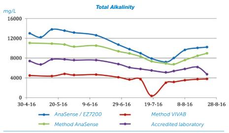
Figure 3: Comparison between the online measurements and the weekly laboratory results at Getteröverket WWTP
