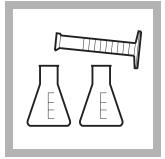
**7.** Add 35 mL of the BoroVer 3/Sulfuric Acid Reagent Solution to each erlenmeyer flask using a 50-mL graduated cylinder. Swirl to mix completely.
