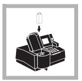
12. Place the prepared sample into the cell holder. Close the light shield. Results in mg/L boron (or chosen units) will be displayed.
