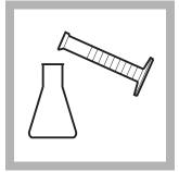
**3.** Measure 75 mL of concentrated sulfuric acid, ACS, using a 100-mL graduated cylinder, into a 250-mL plastic erlenmeyer flask.
