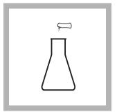
**4.** Add the contents of one BoroVer 3 Reagent Powder Pillow to the flask. Swirl to mix. Allow 5 minutes for the powder to dissolve completely.
