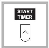
**8.** Press the soft key under **START TIMER**. A 25-minute reaction
