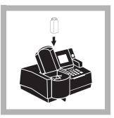
**10.** Place the blank into the cell holder. Close the light shield.
