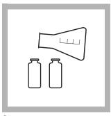
**9.** When the timer beeps, pour at least 10 mL from each flask into separate 1-inch sample cells.
