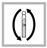
**6.** Hold the vial by the cap over a sink. Invert **gently** 2–3 times to mix. The vial will become **very hot** during mixing.
