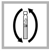
**2.** Invert a few times to bring the sediment into suspension.
