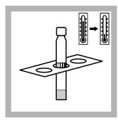
**10.** Place the vial into a rack and **cool** down to room temperature.
