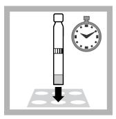
**7.** Place the vial into the **preheated** reactor. Heat in the reactor for **2 hours**.
