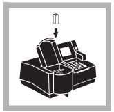
**7.** When prompted, place the sample in the cell holder and close the light shield.
