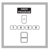
1. Press the soft key under *HACH PROGRAM*. Select the stored program number for tristimulus values by pressing **1666** with the numeric keys.
