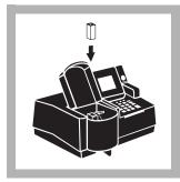
**5.** Insert a 1-cm cell adapter into the cell compartment. Place the blank into the 1-cm adapter. Close the light shield.
