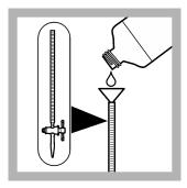
**2.** Fill a 50-mL buret to the zero mark with the titrant.
