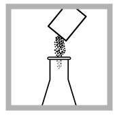
**6.** Add the contents of one Bromphenol Blue Indicator Powder Pillow. The indicator is not necessary if a pH meter is used.
