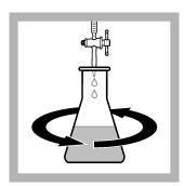
8. Put the flask under the buret. Swirl the flask. Add titrant until the color changes from yellow to pure green (pH 3.7).
