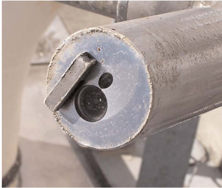
The built-in wiper of the suspended solids sensor prevents measurement error due to fouling
