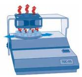
Using TNTplus Vial Tests and the TOC-X5 shaker, the TIC is purged in just 5 minutes – from up to 8 samples simultaneously.
