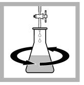
**14.** Put the flask under the buret. Swirl the flask. Add titrant until the color changes from a dark blue to a colorless end point.
