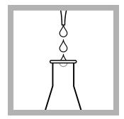
**13.** Add 1 mL of Starch Indicator Solution. A dark blue color develops.
