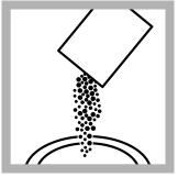
2. Add the contents of one Manganous Sulfate Powder Pillow and one Alkaline Iodide-Azide Reagent Powder Pillow to the sample.
