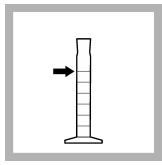
**9.** Pour the prepared sample into a 250-mL graduated cylinder to the 200-mL mark.
