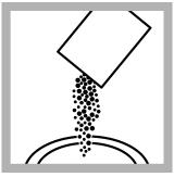
**6.** Remove the stopper and add the contents of one Sulfamic Acid Powder Pillow to the sample.
