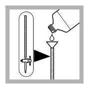
**11.** Fill a 25-mL buret to the zero mark with 0.025 N Sodium Thiosulfate Standard Solution.
