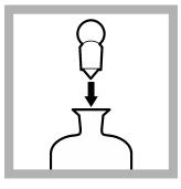
**3.** Immediately put the stopper in the bottle. Make sure that no air is inside the bottle.
