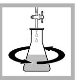
**12.** Put the flask under the buret. Swirl the flask. Add titrant until the color changes yellow to a pale yellow.
