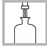
**1.** Collect a water sample in a clean 300-mL BOD bottle. Let the sample overflow the bottle for 2 or 3 minutes to remove trapped air bubbles and to make sure that a representative sample is collected.
