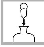
7. Immediately put the stopper in the bottle. Make sure that no air is inside the bottle.
