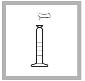
**4.** Add the contents of one ZincoVer 5 Reagent Powder Pillow to the cylinder. Stopper. Invert several times to dissolve the powder completely.
