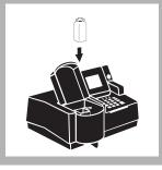
**10.** When the timer beeps, place the blank in the cell holder. Close the light shield.
