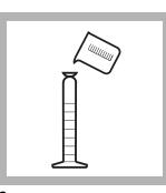
**3.** Fill a 25-mL graduated mixing cylinder with 20 mL of sample.
