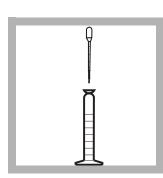
**6.** Add 0.5 mL of cyclohexanone to the remaining solution in the graduated mixing cylinder.
