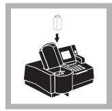
**12.** Place the prepared sample in the cell holder. Close the light shield. Results in mg/L zinc (or chosen units) will be displayed.
