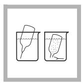
**5.** Fill a PhosVer 3 Phosphate AccuVac Ampul with sample.
