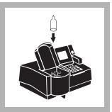
**10.** Place the AccuVac Ampul into the cell holder. Close the light shield. Results in mg/L PO<sub>4</sub><sup>3-</sup> (or chosen units) will be displayed.
