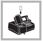
**8.** When the timer beeps, place the zeroing vial into the cell holder. Close the light shield.
