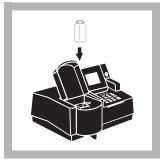
**8.** Place the prepared sample into the cell holder. Close the light shield. Results in mg/L PO<sub>4</sub><sup>3-</sup> (or chosen units) will be displayed.
