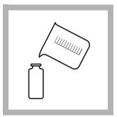
**6.** Fill another sample cell (the blank) with 10 mL of sample. Place it into the cell holder.
