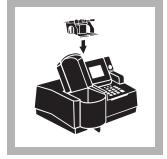
**4.** Insert the AccuVac Ampul Adapter into the sample cell module by sliding it under the thumb screw and into the alignment grooves. Fasten with the thumb screw.
