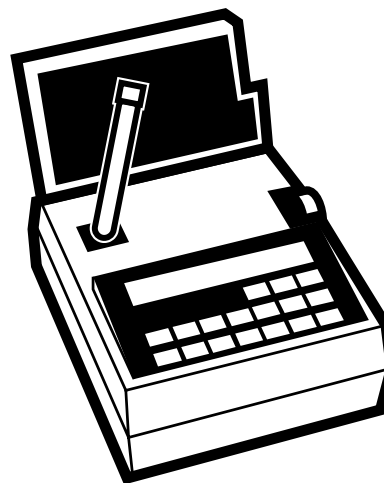
Figure 6. Reading COD results on a DR/2010 Spectrophotometer.
