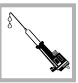
**3.** Hold the Digital Titrator with the cartridge tip up. Turn the delivery knob to eject air and a few drops of titrant. Reset the counter to zero and clean the tip.
