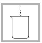
4. If the pH is less than 6 or greater than 7.5, add 1.0 mL of pH 7 Phosphate Buffer Solution to make the prepared sample.
