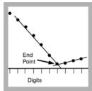
11. Draw the two best intersecting lines through the points plotted as shown above. Determine the number of digits at the intersection of the two lines. This is the end point.
