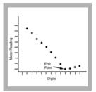
10. Use linear graph paper to plot the recorded readings from the Amperometric Titrator on the vertical axis and the corresponding Digital Titrator digits on the horizontal axis.
