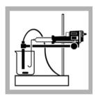
5. Place the beaker on the TitraStir® stand and immerse the tips of both the probe and the delivery tube in the solution. The probe's platinum wires must be submerged. Turn on the stirring motor.
