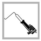
1. Install the 0.00564 N Phenylarsine Oxide (PAO) cartridge. Flush the Digital Titrator delivery tube by turning the delivery knob to eject a few drops of titrant. Reset the counter to zero and wipe the tip.
