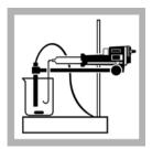
9. Continue the titration, recording at least three points on the downward sloping curve and at least three points after the end point is reached. The latter points will cause little change in the LED readings.
