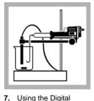
dispense the PAO Titrant Solution in 5 to 10 digit increments while noting the downward reading. If the chlorine content of the sample is high, add titrant at a faster rate.
