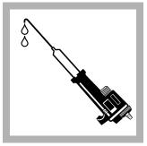
**3.** Hold the Digital Titrator with the cartridge tip up. Turn the delivery knob to eject air and a few drops of titrant. Reset the counter to zero and clean the tip.
