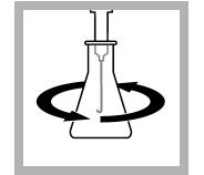
**9.** Put the end of the delivery tube fully into the solution. Swirl the flask. Turn the knob on the Digital Titrator to add titrant to the solution. Continue to swirl the flask. Add titrant until the color changes from yellow to red-brown. Record the number of digits on the counter.
