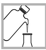
6. If the sample volume is less than 100 mL, dilute to approximately 100 mL with deionized water.
