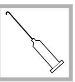
2. Insert a clean delivery tube into the digital titration cartridge. Attach the cartridge to the Digital Titrator. Keep the silver nitrate cartridge in a dark area when not in use.
