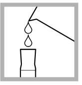
**4.** Use a graduated cylinder or TenSette pipet to measure the sample volume from Table 1 on page 3.
