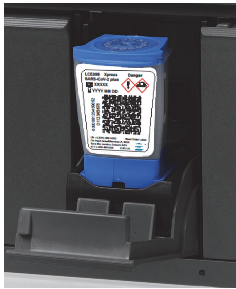
Figure 5-24. GeneXpert Cartridge, Positioned at the Heel of the Module Bay Floor
