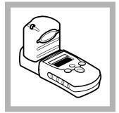
**9.** Install the instrument cap over the cell holder.
