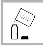
2. Prepare the sample: Fill a sample cell to the 10-mL mark with sample.
