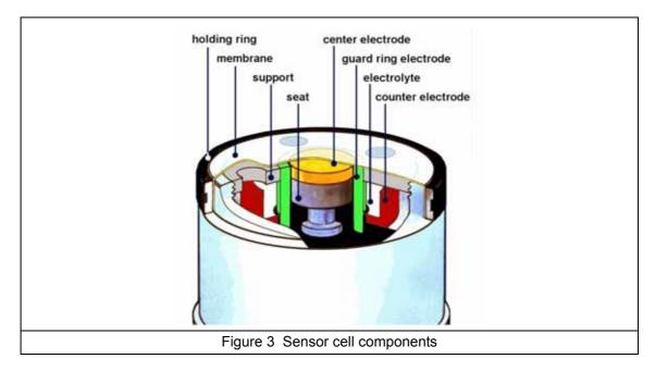
The sensor is designed with one center electrode (cathode) and one counter electrode (anode) immersed in an electrolytic solution. The electrodes and the electrolyte are separated from the gaseous or liquid sample by a membrane permeable to gas.
