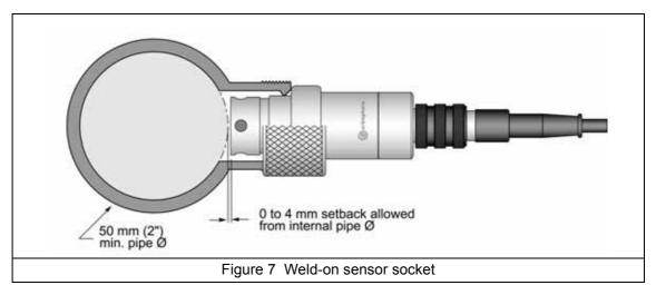
**Note:** Be sure to remove the two O-rings from the socket before welding. Leave the sensor's stainless steel cap screwed on during welding to prevent thread distortion.
