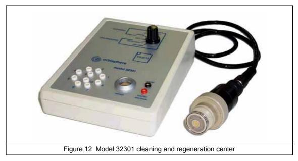
**Note:** It is mandatory to use the 32301 Sensor Cleaning and Regeneration Center for servicing electrochemical H<sub>2</sub> sensors. This process is called dechloridization and rechloridization of the electrodes. See Hydrogen sensor cell cleaning on page 33.
