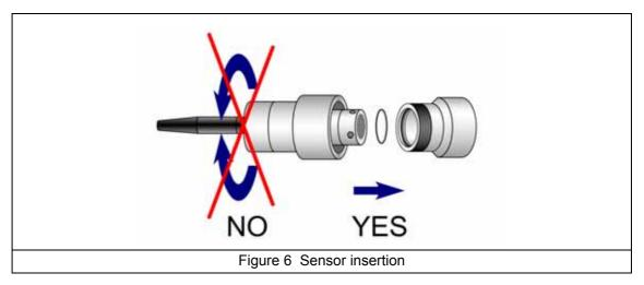
**Note:** Check that the small O-ring at the bottom of the flow chamber is present during removal and installation of the sensor, as it may stick to the sensor head and fall.
