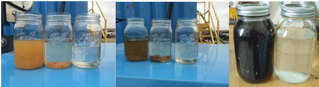
Figure 1: Examples of Produced water (left), flowback (middle), and a side-by-side comparison of recovered oil (right)
