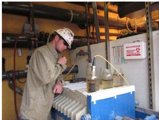
Figure 3: Frac water testing
