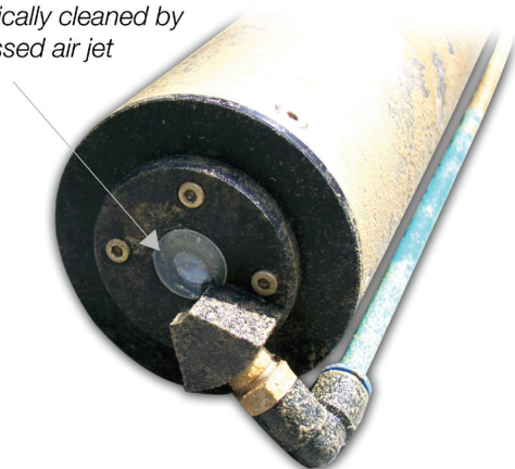
Figure 3. Head of FP 360 sc oil-in-water probe with air blast cleaning system...
