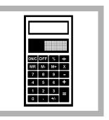
**12.** Use the multiplier in Table 2 on page 3 to calculate the concentration. Digits used × digit multiplier = mg/L total hardness as CaCO<sub>3</sub>
