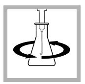
11. Put the delivery tube point fully into the solution and swirl the flask. Turn the knob on the Digital Titrator to add titrant to the solution. Continue to swirl the flask and add titrant until the color changes from red to pure blue. Record the number of digits on the counter.
