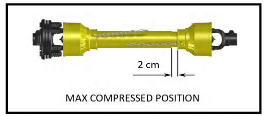
A driveshaft too long may cause structural damages to the tractor and machine. If the driveshaft is too long, it may be adapted by removing it and shortening the tubes according to the instructions provided by the manufacturer in its use and maintenance manual.
