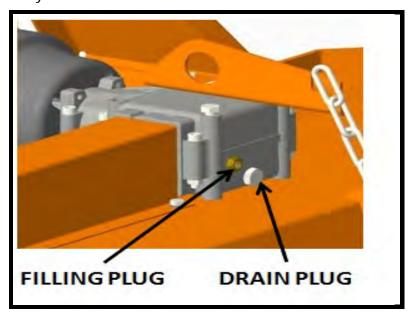
If the sign is below the minimum, fill up oil till restore the correct level.
