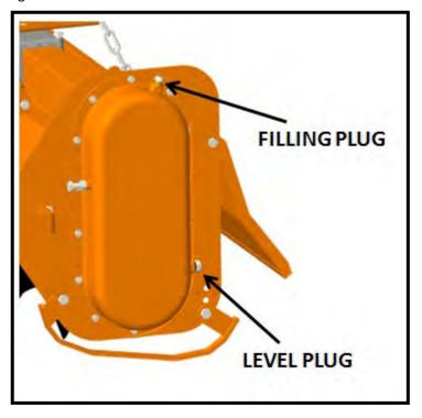
Check the oil level every 50 hours, making sure it reaches the level plug on the transmission cover. If the oil is below this level, fill up oil till restore the level.
