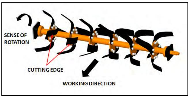
Periodically check the tightness of screws and nuts, and tighten if necessary.
