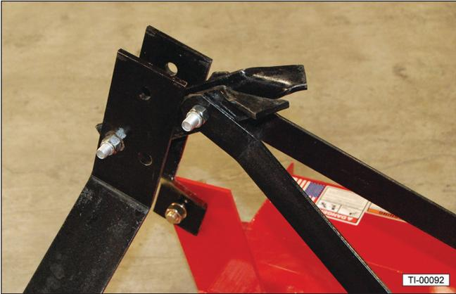
10. Remove the four 5/16-18 x 1/2" bolts from the front of the gearbox.
