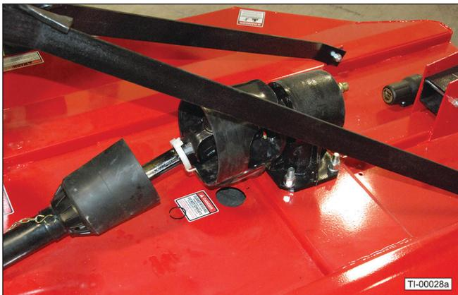
16. Install 1/2-13 x 3" Grade 2 shear bolt (11) and lock nut (12). Install the snap ring in the groove on the input shaft (shown by arrow).
