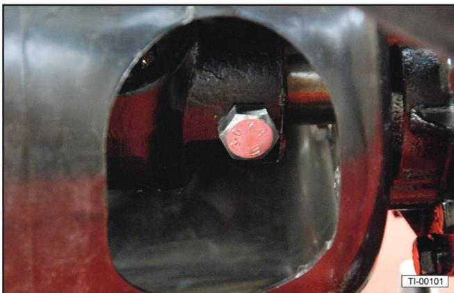
2. Rotate the driveline to align shear bolt with the access hole in the gearbox shield. Remove the
