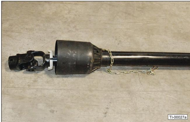
15. Slide the driveline onto the gearbox input shaft. Align the shear bolt holes in the shaft and the U-joint.
