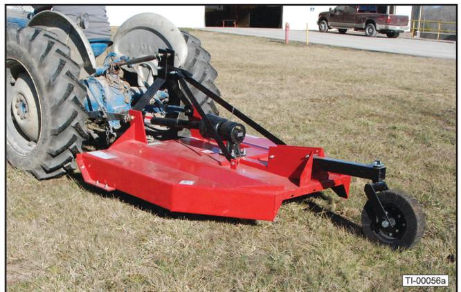
5. Large, dense, or wet vegetation may need to be cut in two or more passes to achieve a uniform cut. In such conditions, raise the cutting height to 12" or more on the first pass. Then lower the rotary cutter to the desired height and mow the vegetation a second time. If possible, select a cutting direction that is at a 90 degree angle to the first pass to reduce streaking for a more uniform cut.
