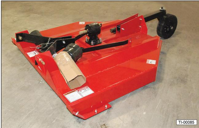
6. Cut the wires holding the driveline parts to the A-frame. Set the driveline aside for now.
