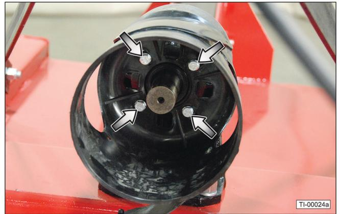
13. Separate the two halves of the driveline.
