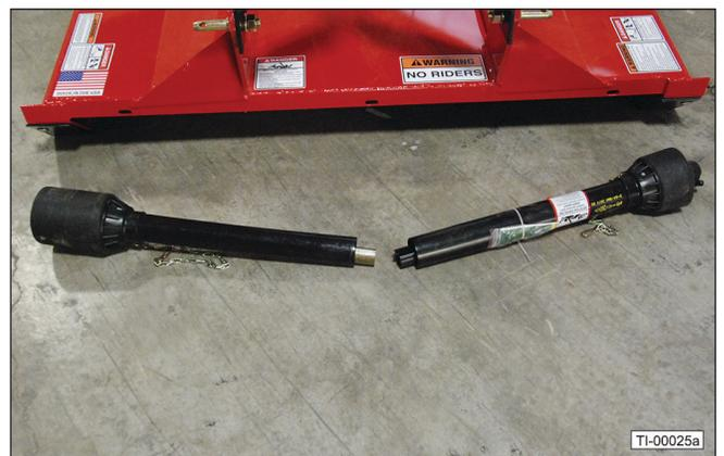
14. Depress the tab on the implement end of the driveline and slide the outer shield down and away from the U-joint.
