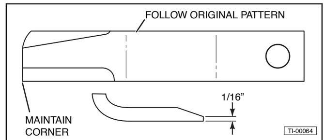
Replace the blades when worn more than 1/2" from the original edge. Always replace blades in pairs.
