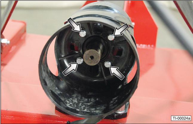
19. Separate the two halves of the driveline.
