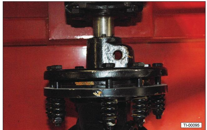
22. Install the retaining bolt and tighten the locknut.
