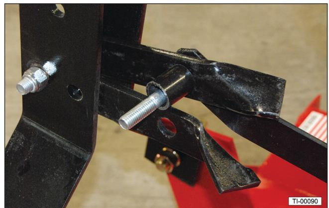
9. Tighten the bolt sufficiently to eliminate side play, but still allow the break link to function.
