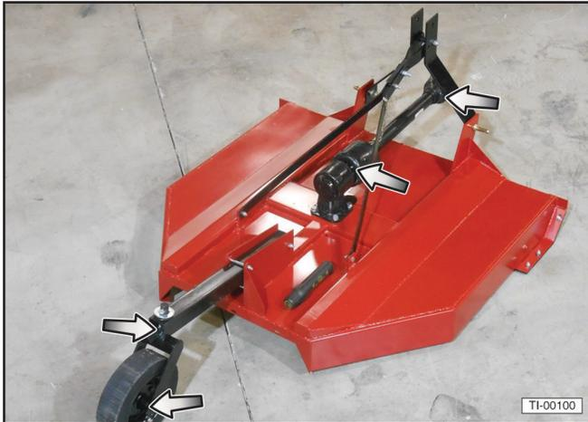
Grease all zerks every fifty hours of operation. Use an SAE multipurpose high-temperature grease with extreme pressure (EP) performance. Also acceptable is an SAE multipurpose lithium base grease.
