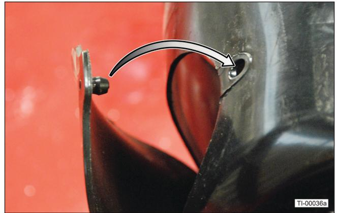
24. Slide the front driveline half over the rear half. Align the square rib on the mating halves to engage.
