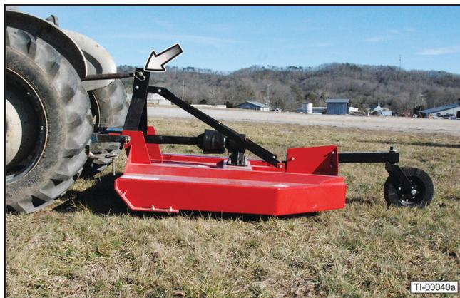
4. Disconnect the lift arms and remove the rotary cutter driveline from the tractor PTO shaft. Lay the driveline down carefully to avoid damaging the driveline or its shield. Do not let the driveline fall into mud or dirt, which can contaminate the bearing and shorten the life of the driveline.
