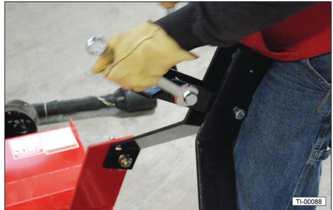
8. Position the back braces on the outside of the break link and reinstall the bolt. Be sure the spacer is in place.
