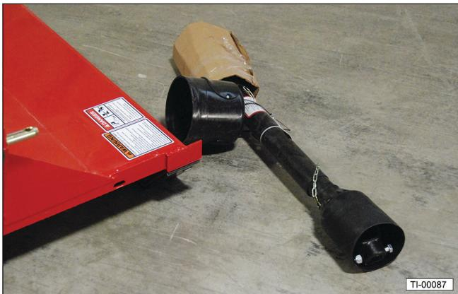
7. Stand the A-frame up and remove the 5/8-11 x 4-1/2" bolt, locknut, and spacer on the break link.
