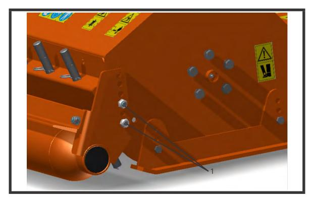
Depending on the different roller positions, it is possible to set four different cutting heights: 32-57-82 and 107 mm.
