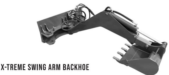
Our X-treme Swing Arm Backhoe is an excellent tool for digging ditches, removing stumps and digging footings. It uses an electric over hydraulic control to operate both the bucket and swing cylinder from one auxiliary valve on your machine. This allows a 110 degree swing right or left.
