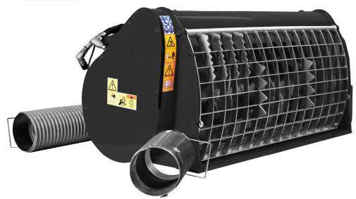
The BMX-100, 250, 450, and 600 mixers make up the line of the Mix & Go Skid Steer Concrete Mixers. Capacities range between 3.34 cu. ft. and 21 cu. ft. allowing them to fit a variety of machine sizes and operations. All models can handle aggregate of up to 1.25" in diameter. Each size mixer seamlessly scoops, mixes, and dispenses a variety of cementitious materials.
