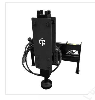
The IronCraft Post Driver is a dependable post driving attachment for operators looking to get the job completed in a timely manner for an excellent cost. These breaker style post drivers use a proven nitrogen charged power cell, steel plate frame, and high strength steel domed head to put posts in the ground in a fraction of the time it takes to set posts with a conventional post hole digger. Offered in the skid steer or excavator mounts, ready to go when received.
