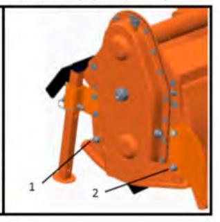
When finished, verify that both skids are at same level, and check if the front of the tiller is leveled to the back, when lowered to the ground. Adjust with the 3-point top link if necessary.
