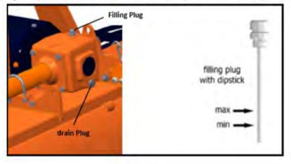
If the sign is below the minimum, fill up oil till restore the correct level.
