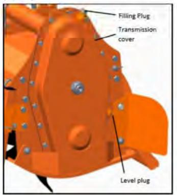
Check the oil level every 50 hours, making sure it reaches the level plug on the transmission cover.
