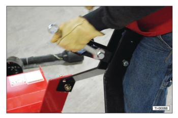
8. Position the back braces on the outside of the break link and reinstall the bolt. Be sure the spacer is in place.
