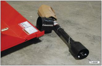
Stand the A-frame up and remove the 5/8-11 x 4-1/2" bolt, locknut, and spacer on the break link.
