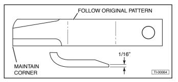
Replace the blades when worn more than 1/2" from the original edge. Always replace blades in pairs.
