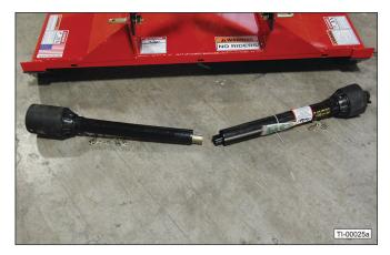
20. Remove the retaining bolt from the slip clutch.
