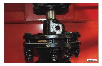
22. Install the retaining bolt and tighten the locknut.
