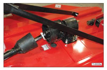
16. Install 1/2-13 x 3" Grade 2 shear bolt (11) and lock nut (12). Install the snap ring in the groove on the input shaft (shown by arrow).
