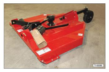
6. Cut the wires holding the driveline parts to the A-frame. Set the driveline aside for now.
