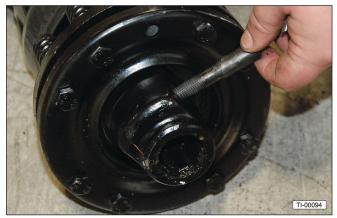
21. Line up the spline grooves and slide the slip clutch onto the gearbox input shaft until the retaining bolt hole aligns with the groove in the shaft.
