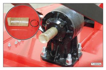
12. Position the driveline shield on the front of the gearbox and re-install the bolts.
