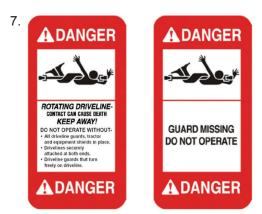
**ROTATING DRIVELINE HAZARD** KEEP AWAY Do not operate unless PTO guards, tractor master shield and implement guards are in place. PTO guards must turn freely and be properly attached and maintained. U-joint yokes must be securely locked onto tractor and implement shafts. Be sure tractor drawbar and implement hitch are adjusted correctly. Grease shaft regularly. This implement is designed to operate at 540 RPM maximum tractor PTO speed. Failure to heed these warnings may result in
