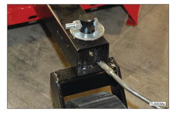
29. Apply grease to the zerk on the tailwheel hub.
