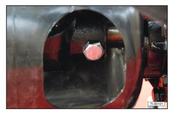
2. Rotate the driveline to align shear bolt with the access hole in the gearbox shield. Remove the
