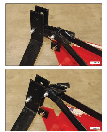
10. Remove the four  $5/16-18 \ge 1/2$ " bolts from the front of the gearbox.
