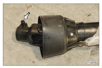
3. Push the driveline onto the tractor PTO shaft until the locking pin engages.
