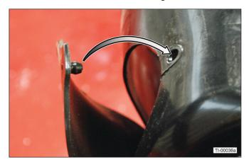
27. Attach the chain on the outer shield to the rotary cutter.
