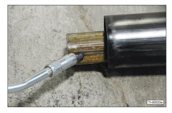
24. Slide the front driveline half over the rear half. Align the square rib on the mating halves to engage.
