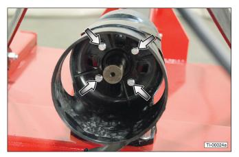
19. Separate the two halves of the driveline.
