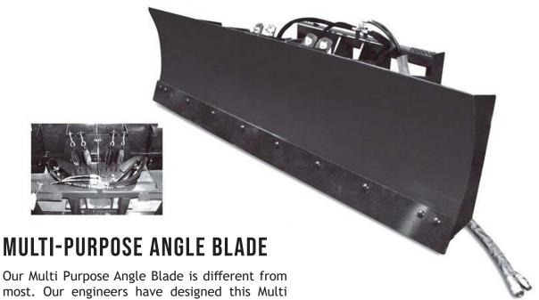
Our Multi Purpose Angle Blade is different from most. Our engineers have designed this Multi Purpose Angle Blade to be used as a snow plow and a angle blade with ease. To use this as a snow plow, simply remove the center pin. This allows the blade to tip when hitting something. Our powerful springs retract the blade into position as soon as the object is cleared.
