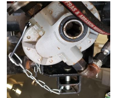
5.4B CHAIN TORQUE BAR IS AT APPROX. 90°
