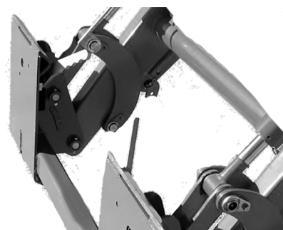
FIGURE 3.2C TRACTOR PIN ON HOOKUP
