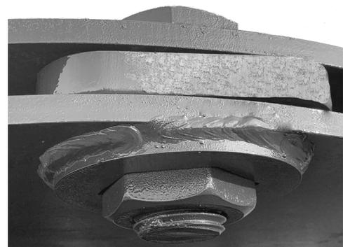
Figure A3 Bolt Head Bead Weld & Assembly
