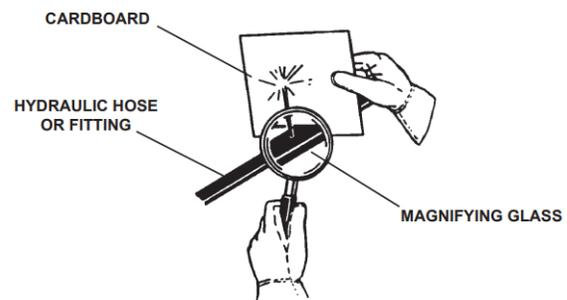
5. Inspect the excavator cutter hydraulic plumbing for noticeable leaks. Fix before continuing.
