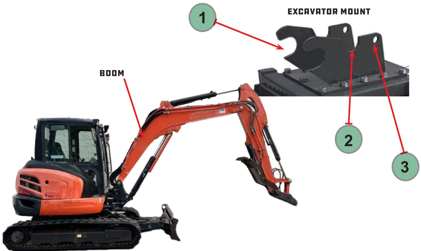
FIGURE 3.2A - EXCAVATOR QUICK ATTACH COUPLER TO EXCAVATOR MOUNT
