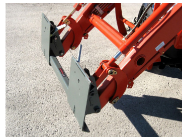
FIGURE 4.2D TRACTOR PIN ON HOOKUP
