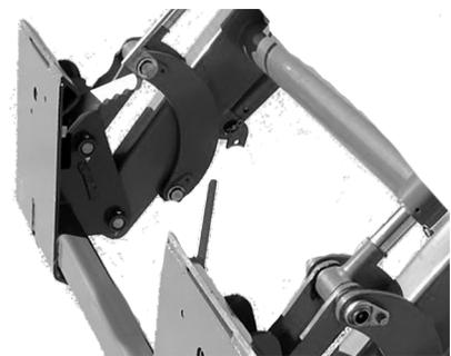
**FIGURE 4.2C TRACTOR PIN ON HOOKUP**
