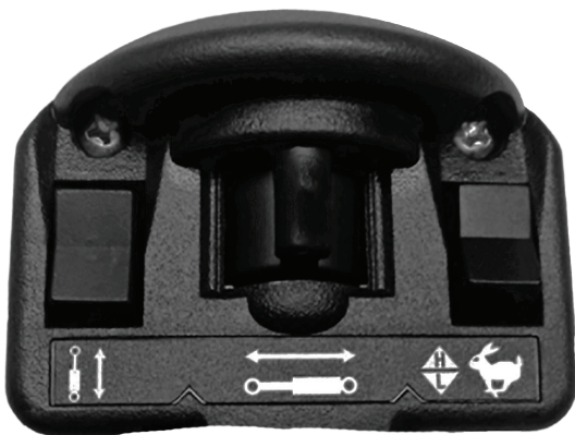
Typical Machine Auxiliary Electric Controller
