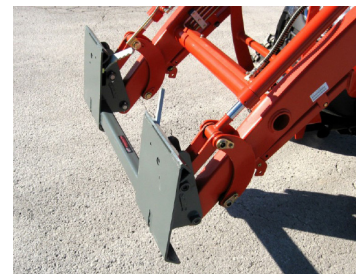
FIGURE 4.2C TRACTOR PIN ON HOOKUP
