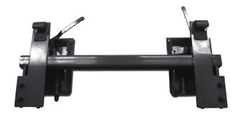
Your pin on tractor can easily be converted to a skid steer quick attach. All we require are a few simple measurements. For those that have John Deere loaders or Euro loaders, we also make a conversion to attach to your loader which enables you to use skid steer attachments.
