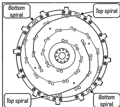
PermaBond A134, Loctite 635 or equivalent in each SURFACE TOOTH HOLDER corre-
