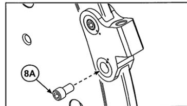
21. Finally torque all the SOC. HEAD BOLT 5/8-18 x 1 1/4" according to "Disc part nomenclature & torque specification" on page 42.
