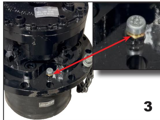
9. Lay the Bearing Housing on its side with the oil ports facing up. See Example 4
