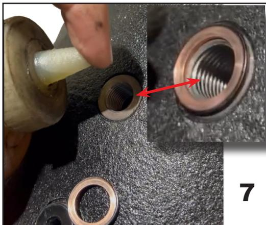
15. Place the washer and oil port bolt on the BOTTOM PORT and tighten tightly with an Allen wrench. **See Example 8a & 8b**
