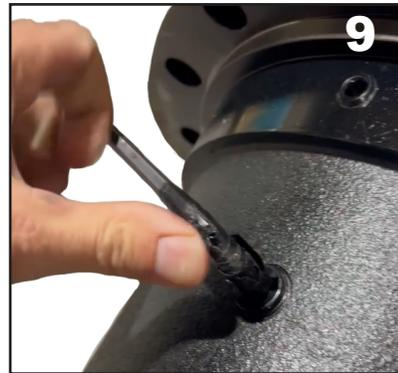
19. Tighten the air port on top of the motor. **See Example 10**
