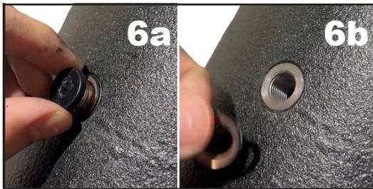
12. Stand the Bearing Housing up and allow the oil to drain from the port holes. (You may need to tilt the Bearing Housing to fully empty.)
