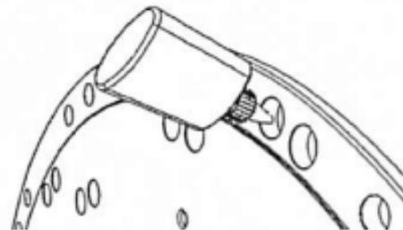
5. Then equally spread the bond all around the internal area of the hole with your finger.
