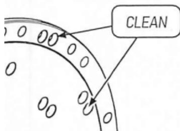
4. Starting with PERIPHERAL TOOTH HOLDER mounting holes, apply a retaining compound such as Permabond A134, Loctite 635, or equivalent into each PERIPHERAL TOOTH HOLDER corresponding disc hole. Spread the
