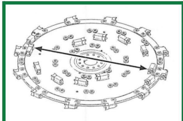
Always replace two tooth holders of equal weight and install them 180° opposite to each other on the disc to prevent an unbalancing situation of the disc. Always use new cap screws and sleeves when replacing them.
