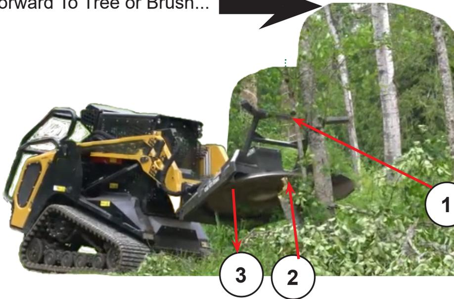
Use the push bar to push the tree while cutting to prevent it falling back on the host machine..
