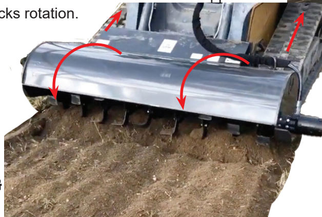
FIGURE 3.5B CORRECT TILLER TINE ROTATION & MACHINE DIRECTION.
