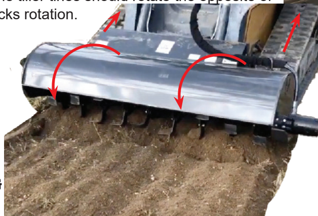
FIGURE 3.5B CORRECT TILLER TINE ROTATION & MACHINE DIRECTION.
