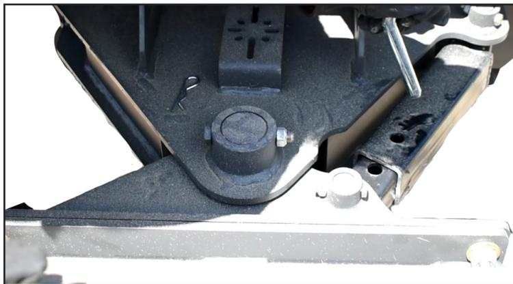
FIGURE 4.6C ANGLE CHANGE LOCKING PIN
