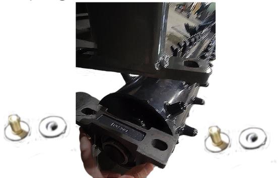
8. Place another washer on the screw and finger tighten the locknut. **Figure 5.5D**
