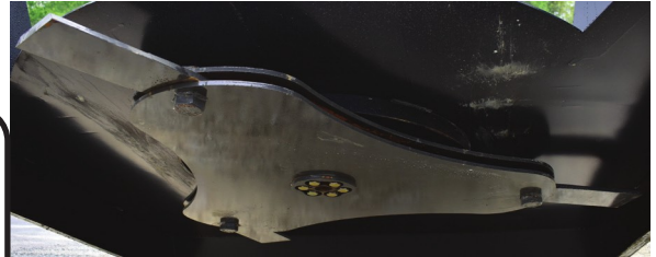
Blade Holder Without Mulching Teeth- Example
