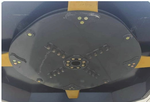
Blade Holder With Mulching Teeth- Example
